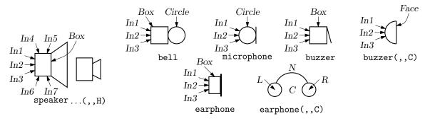
Figure 25: Audio components: speaker(U|D|L|R|degrees, size, type), bell, microphone, buzzer, earphone, with their internally named positions and components.
