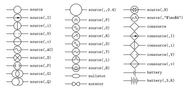
Figure 8: Sources and source-like elements.
