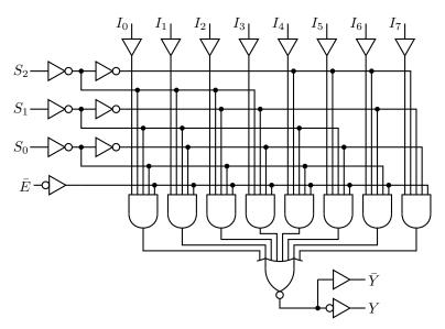
Figure 48: Eight-input multiplexer, showing a gate with wings.
