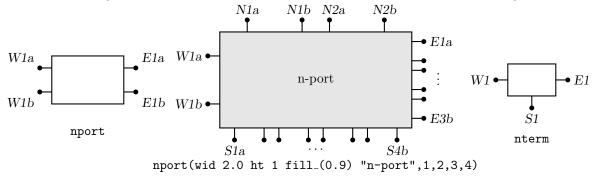
**Figure 26:** The nport macro draws a sequence of pairs of named pins on each side of a box. The pin names are shown. The default is a twoport. The nterm macro draws single pins instead of pin pairs.
