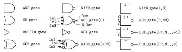
Figure 46: Basic logic gates. The input and output locations of a three-input NOR gate are shown. Inputs are negated by including an N in the second argument letter sequence. A B in the second argument produces a box shape as shown in the rightmost column, where the second example has AND functionality and the bottom two are examples of exclusive OR functions.
