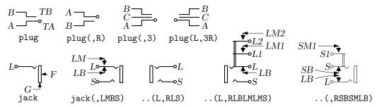
Figure 31: The jack(U|D|L|R|degrees, chars) and plug(U|D|L|R|degrees, [2|3][R]) components and their defined points.
