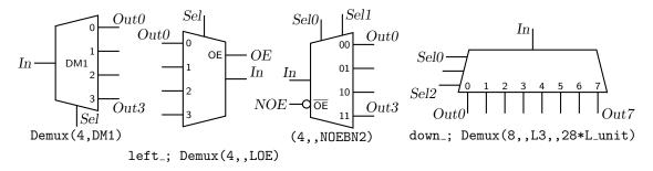
Figure 51: The Demux(input count, label, [L] [B|H] [N[n] | S[n]] [[N] OE], wid, ht) macro.
