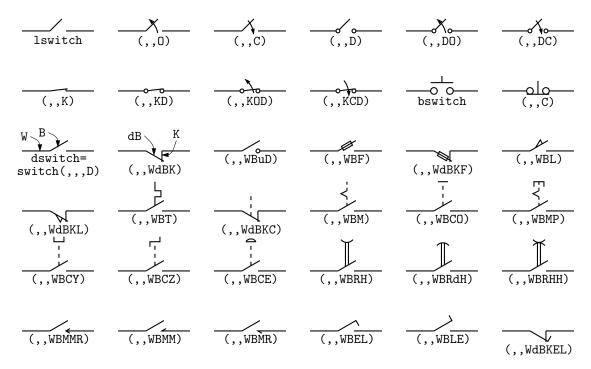
Figure 12: The switch(linespec, L|R, chars, L|B|D) macro is a wrapper for the macros lswitch(linespec, [L|R], [0|C][D][K]), bswitch(linespec, [L|R], [0|C]), and the many-optioned dswitch(linespec, R, W[ud]B[K] chars) shown. The switch is drawn in the current drawing direction. A second-argument R produces a mirror image with respect to the drawing direction.
