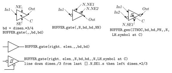
Figure 49: The BUFFER\_gate and BUFFER\_gen macros. The bottom two examples show how the gate can be drawn as a two-terminal macro but internal block locations must be referenced using last [].
