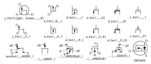
**Figure 42:** JFET, insulated-gate enhancement and depletion MOSFETs, and simplified versions. These macros are wrappers that invoke the mosfet macro as shown in the bottom row. The two lower-right examples show custom devices, the first defined by omitting the substrate connection, and the second defined using a wrapper macro.
