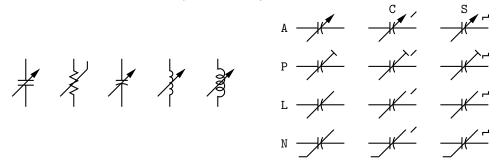
Figure 13: Illustrating variable('element', [A|P|L|[u]N][C|S], angle, length). For example, variable('capacitor(down\_dimen\_)') draws the leftmost capacitor shown above, and variable('resistor(down\_dimen\_)', uN) draws the resistor. The default angle is 45°, regardless of the direction of the element. The array on the right shows the effect of the second argument.
