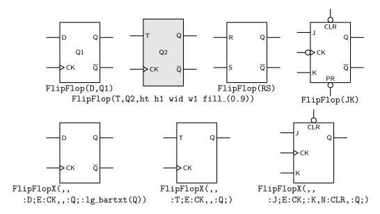
Figure 52: The FlipFlop and FlipFlopX macros, with variations.
