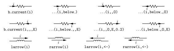
Figure 15: Illustrating b\_current, larrow, and rarrow. The drawing direction is to the right.
