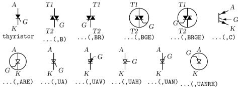
Figure 40: The thyristor(linespec, chars) macro, drawing direction down. The element is not two-terminal, so the linespec determines length and direction but not position. The scr macro places the thyristor as a two-terminal element.
