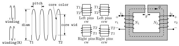
Figure 28: The winding(L|R, diam, pitch, turns, core wid, core color) macro draws a coil with axis along the current drawing direction. Terminals T1 and T2 are defined. Setting the first argument to R draws a right-hand winding.
