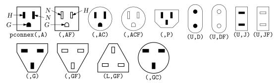
Figure 34: A small set of power connectors drawn by pconnex(R|L|U|D|degrees, chars). Each connector has an internal H, N, and where applicable, a G shape.
