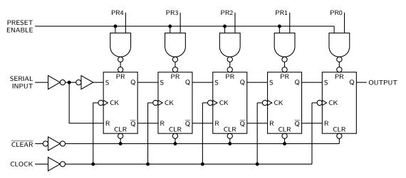
Figure 53: A 5-bit shift register.
